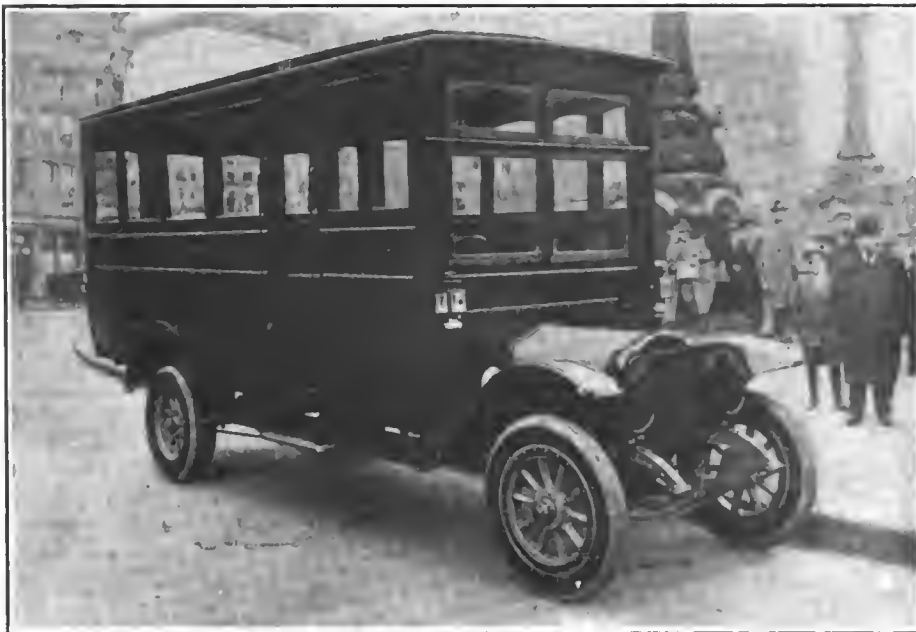
Type of pay-enter motor bus made by the White Company for Indianapolis company
